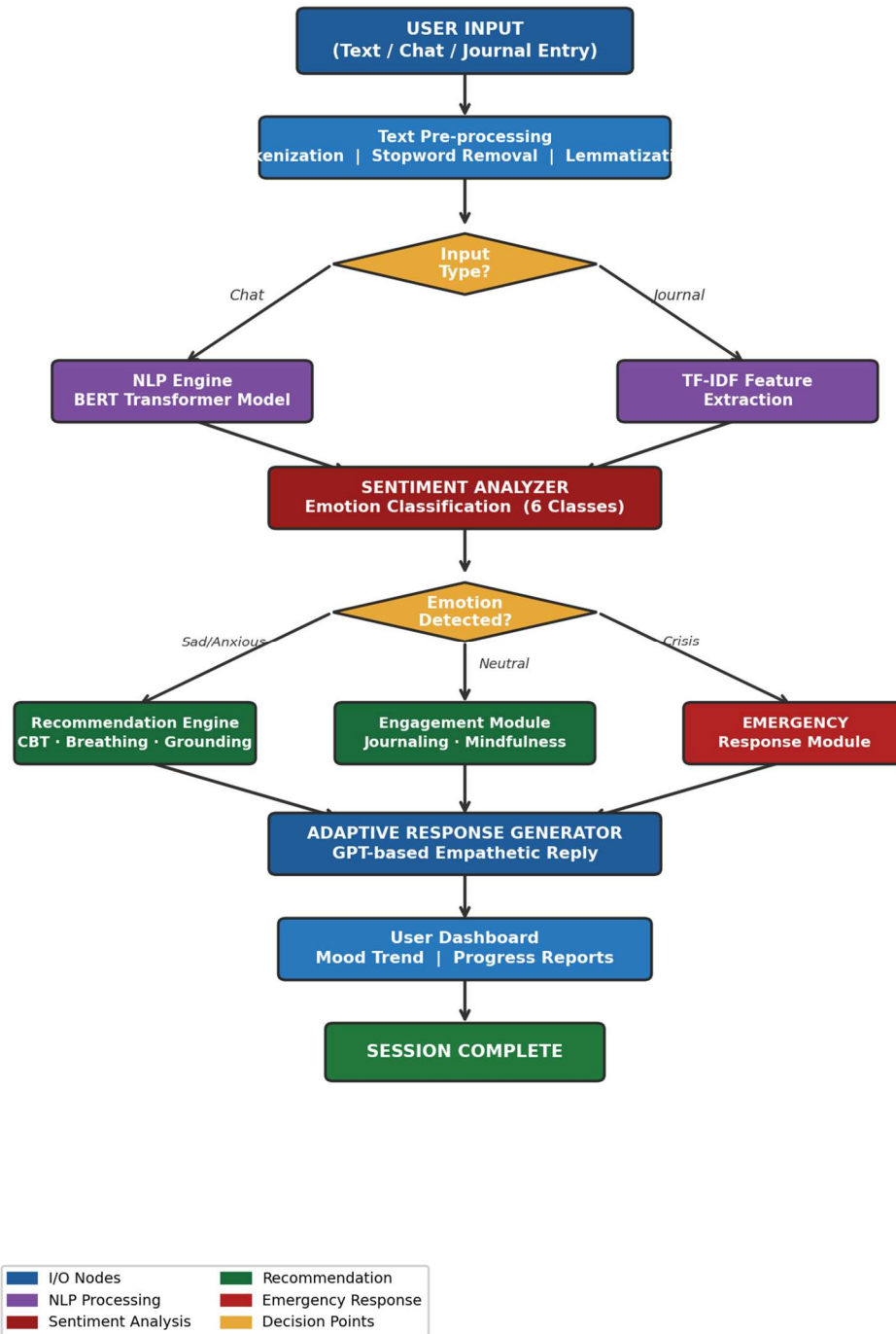
Fig. 4: MindMitra System Architecture and NLP Processing Pipeline Flowchart
